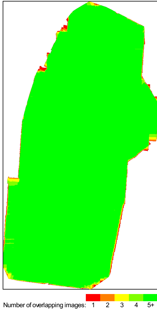
Figure 4: Number of overlapping images computed for each pixel of the orthomosaic. Red and yellow areas indicate low overlap for which poor results may be generated. Green areas indicate an overlap of over 5 images for every pixel. Good quality results will be generated as long as the number of keypoint matches is also sufficient for these areas (see Figure 5 for keypoint matches).
